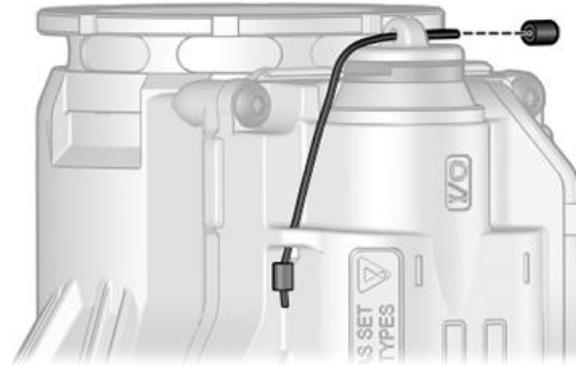
4. Slide a second metal sleeve about 1/16” over the free end of the wire lanyard and use pliers to crimp in place.
